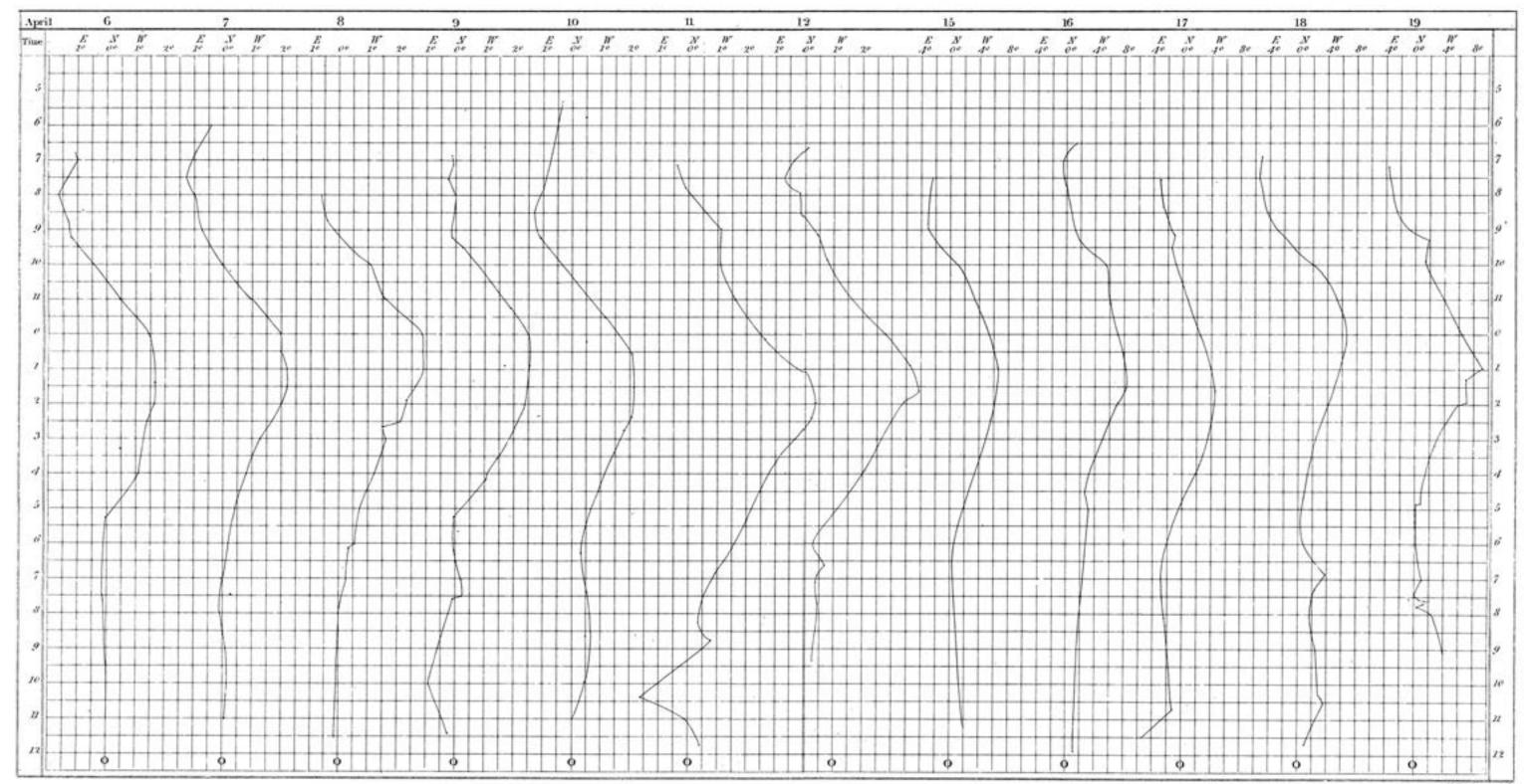
Curves of the diarnal deviations of a magnetic needle whose directive power was diminished by the action of two bar magnets placed in the line of the dip: the N.end of the needle pointing north.
