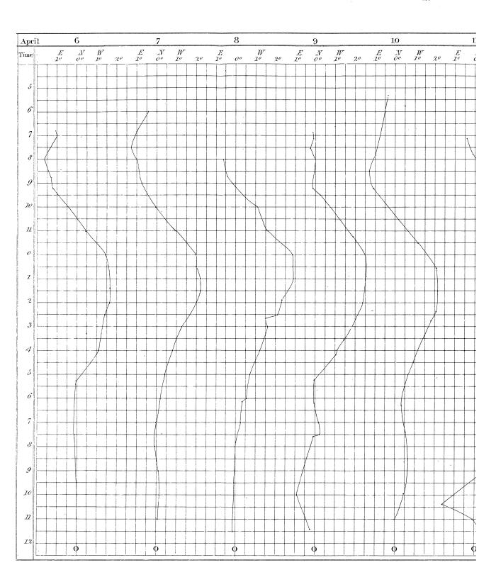
of a magnetic needle whose directive power was diminished by veed in the line of the dip: the N.end of the needle pointing north.
