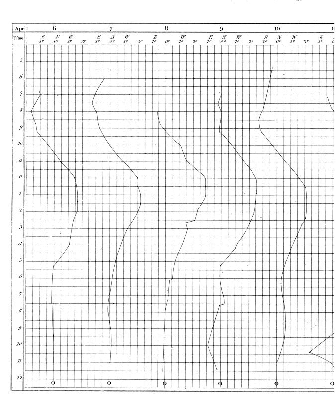
of a magnetic needle whose directive power was diminished by weed in the line of the dip: the N.end of the needle pointing north.
